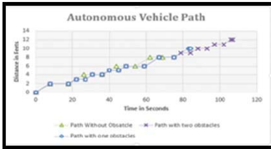
Figure 6.8 Graph of Distance versus time of autonomous vehicle on predefined path
