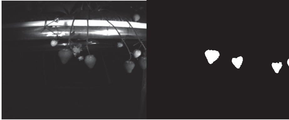
Figure 6: The detection of ripen strawberries by machine vision
