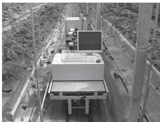
Figure 5: The strawberry-harvesting robot
