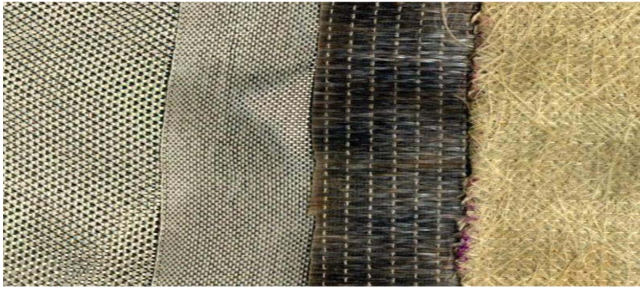
Fig.1 Different types of fiber sheets. (from left Aramid, Basalt, Carbon, Coir)
