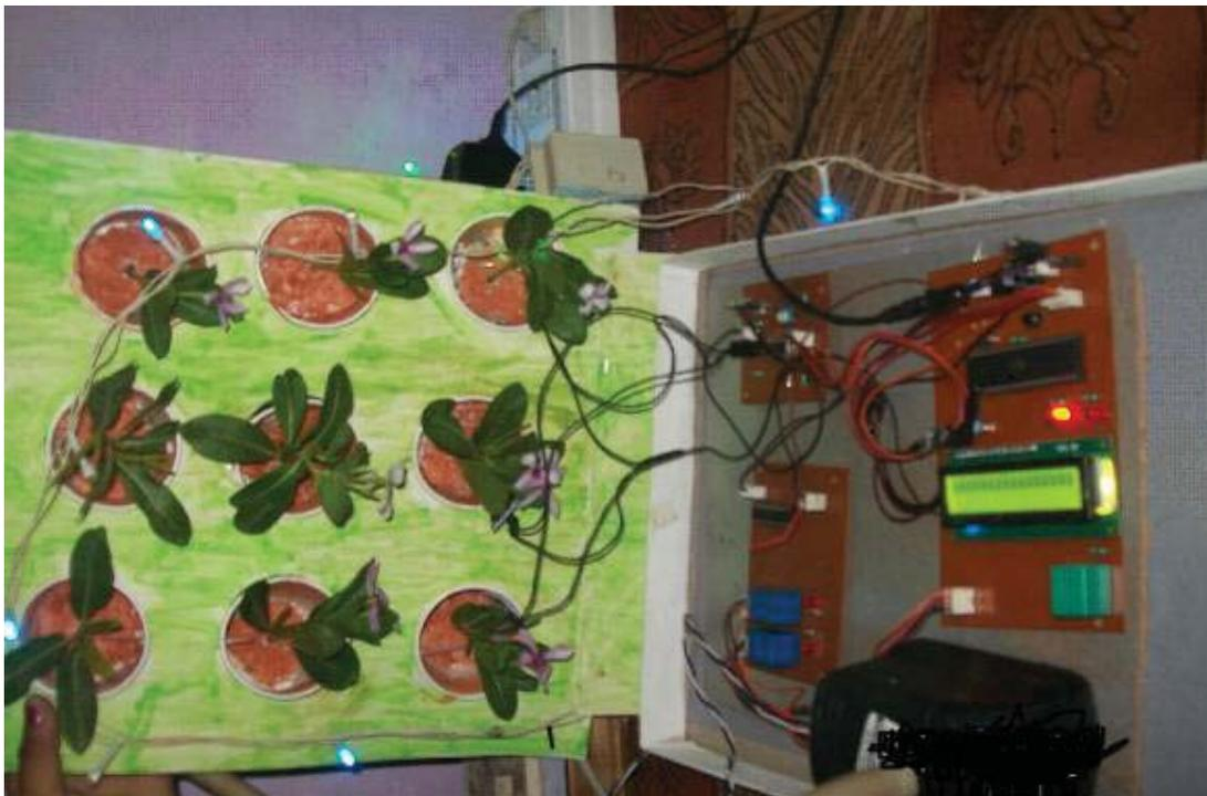
Fig 4 Image of green wall automation system.
