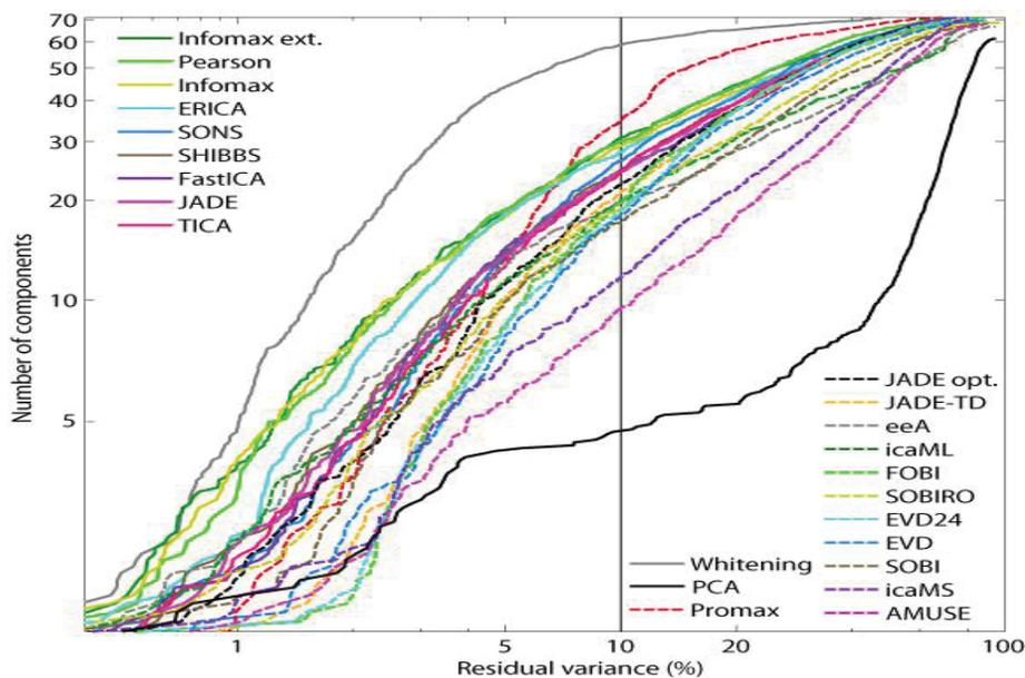
Fig. 1. Number of bipolar component returned as a function of residual variance for each algorithm. Since there were 71 channels in each data set, the ordinate indicates the cumulative number of components at each residual variance. The algorithms are ranked according to their intersection with the vertical line at 10% of residual variance (see Table 1).
