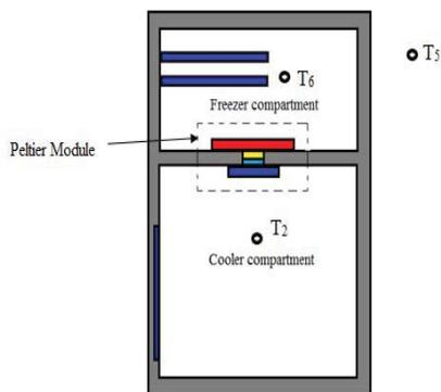
Figure 3 Experimental setup in Structure I
