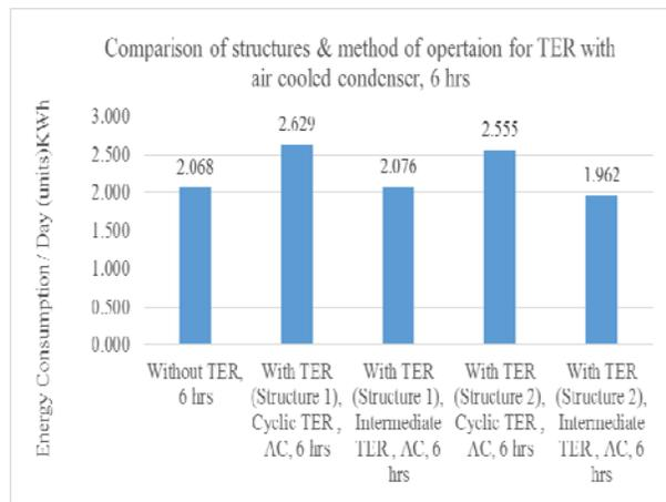
Figure 6 Energy Consumption with different methods with Air cooled
