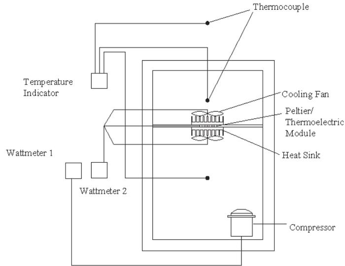
Figure 1 Schematic Diagram of Experimental setup (Front view)
