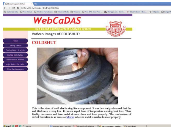
Figure. 6: Information of casting defect – coldshut
