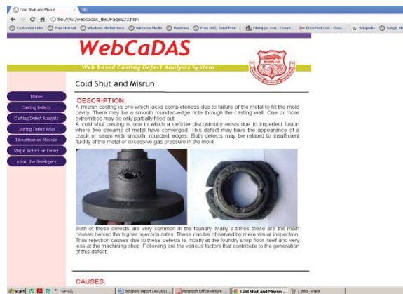
Figure. 6: Information of casting defect – coldshut
