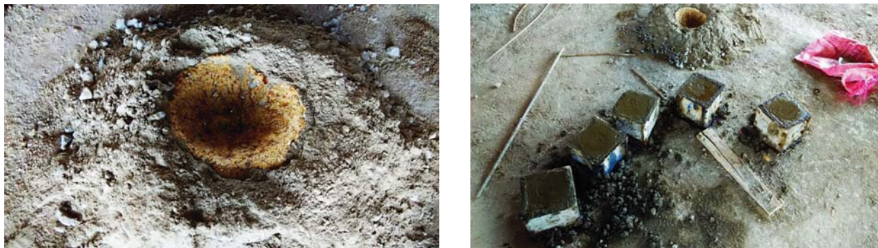
Figure 1: Casting of cubes
