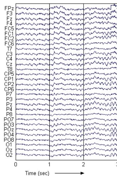
Figure 7 : Corrected EEG i.e., Eye Movement Artifact Removed ( Example 2 )
