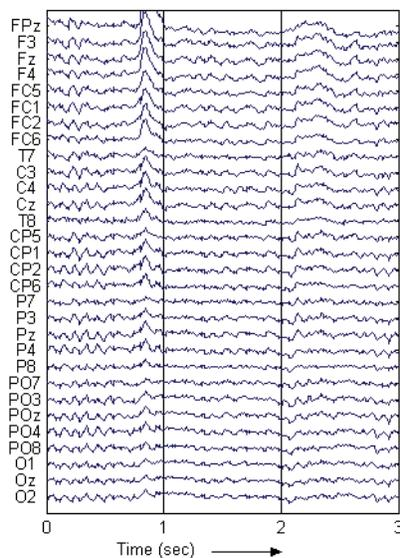
Figure 2 : Original EEG contaminated with EOG (Example 1)
