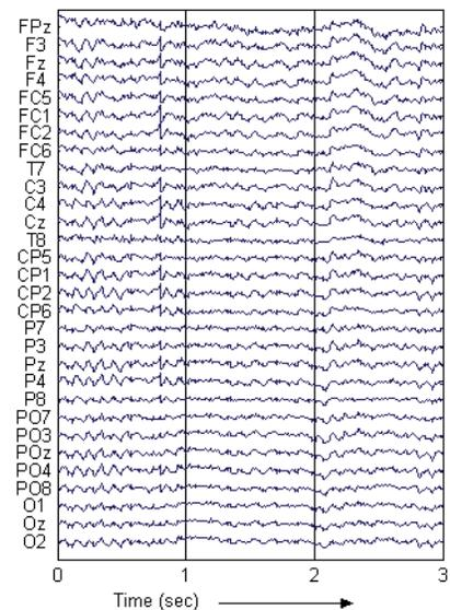
Figure 4 : Corrected EEG i.e., EOG artifact removed (Example 1)
