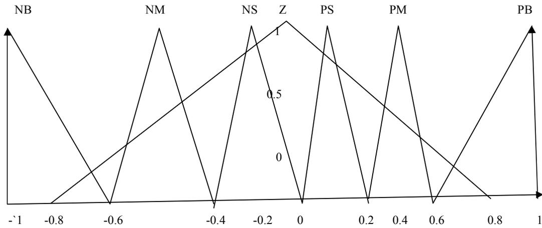
Figure 2(d) output membership function
