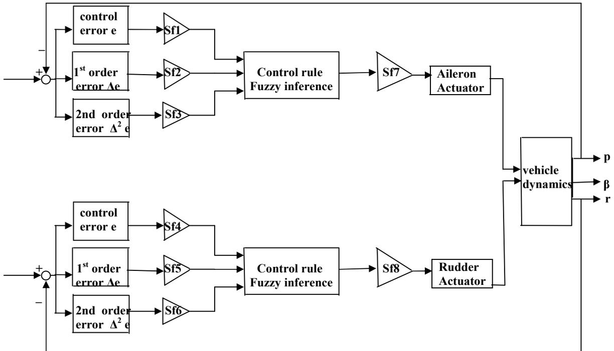
Fig. 1. Block diagram of Fuzzy control law for stability augmentation system
