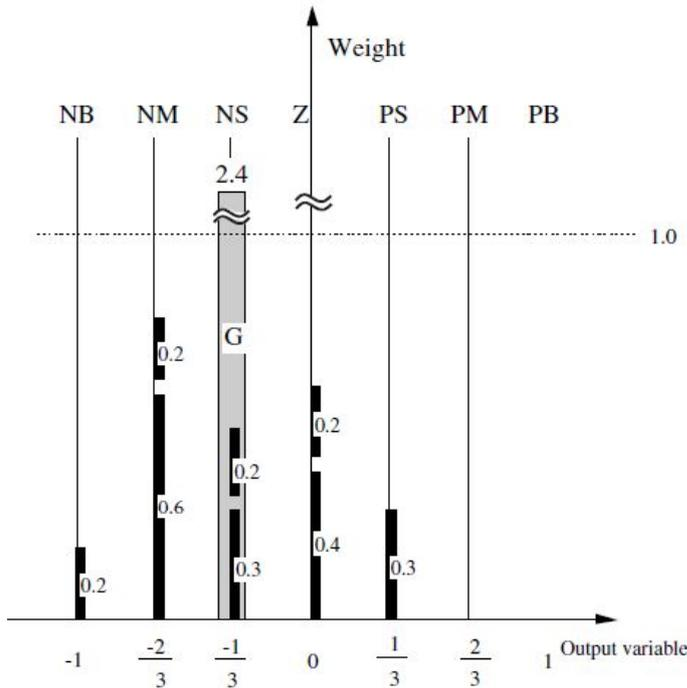
Fig. 5. Computation of center of gravity position.
