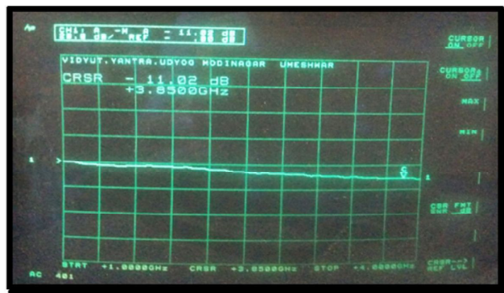
Fig 4:- Network analyzer tested result of 3-pole microstrip low pass filter.
