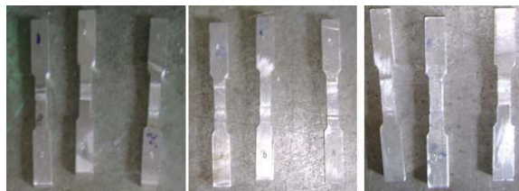
Figure 10.1: Tensile test specimens before testing
