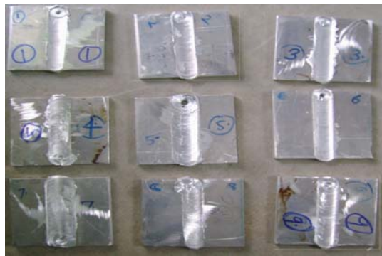
Figure 9.1 Friction stir welded pieces for all 9 experiments
