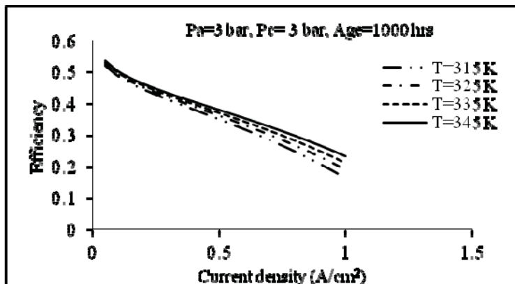
Fig.14 Efficiency as a function of current density at various temperatures
