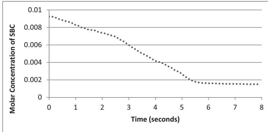
Figure 5. Variation of molar concentration of SBC with time along the pathline trajectory
