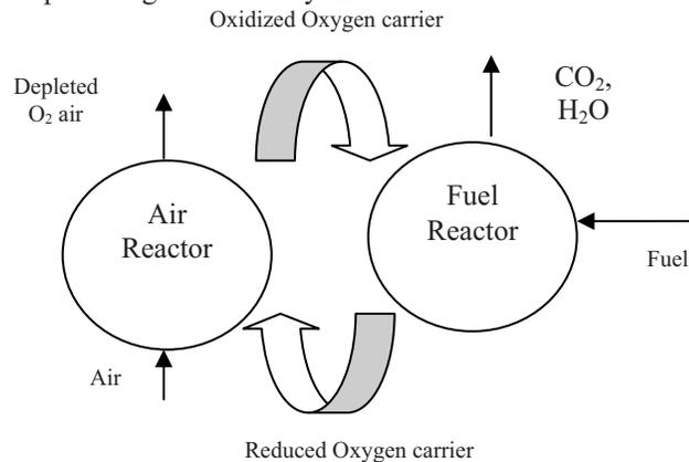
Figure 1. Chemical looping process
