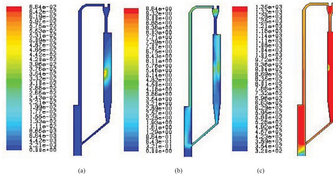
Figure 3. (a) Contour of rate of reaction 1 (b) Velocity profile (c) Temperature profile
