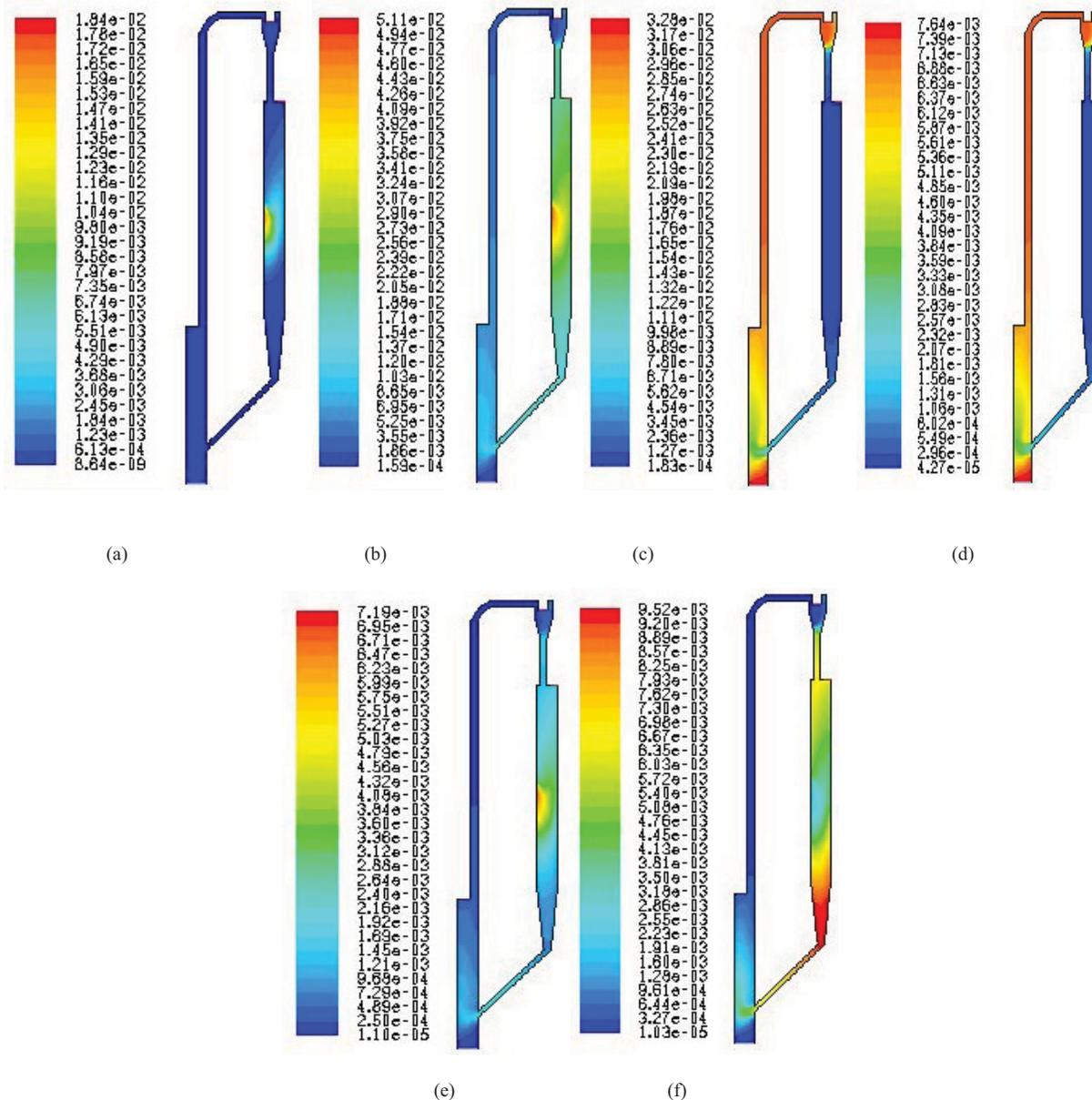
Figure 4. Molar Concentration contour of (a) SBC (b) iron (III) oxide (c) Nitrogen (d) Oxygen (e) carbon dioxide (f) carbon monoxide
