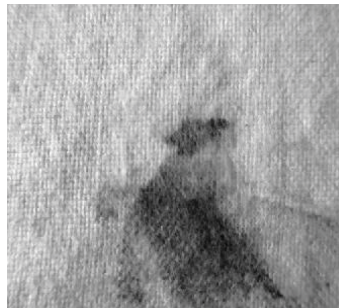
(b) Stain defect woven fabric image
