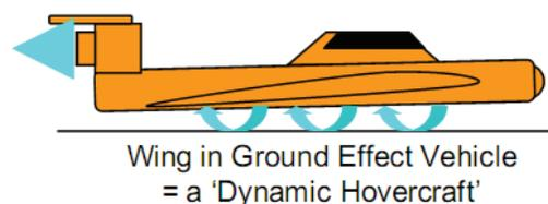
Figure 3: The WIG - a 'dynamic' hovercraft, without skirt or lift engines
