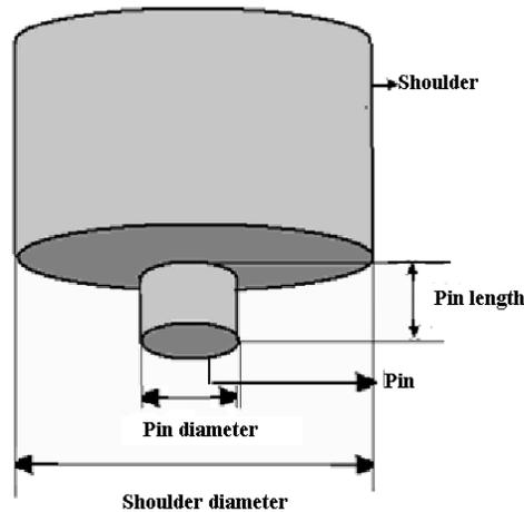
Figure 2. Tool Geometry
