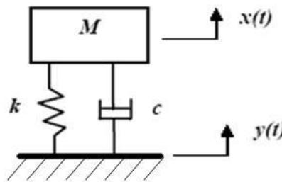
Figure 1. Seismically excited spring-mass-damper system
