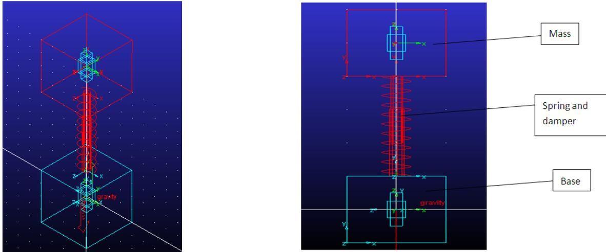
Figure 3. Three dimensional and two dimensional view of the spring-mass-damper system (simulation model)
