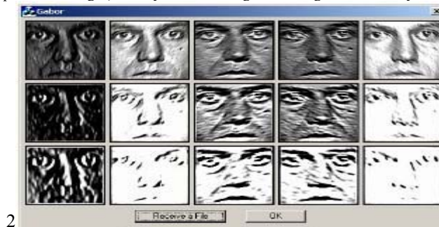
Fig. 4: Gabor filter response of a typical face image (courtesy 'on face recognition using Gabor filter by AI-Amin Bhutiyani and Chang Hung Liu)
