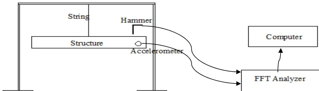
Figure 18. Experimental Setup
