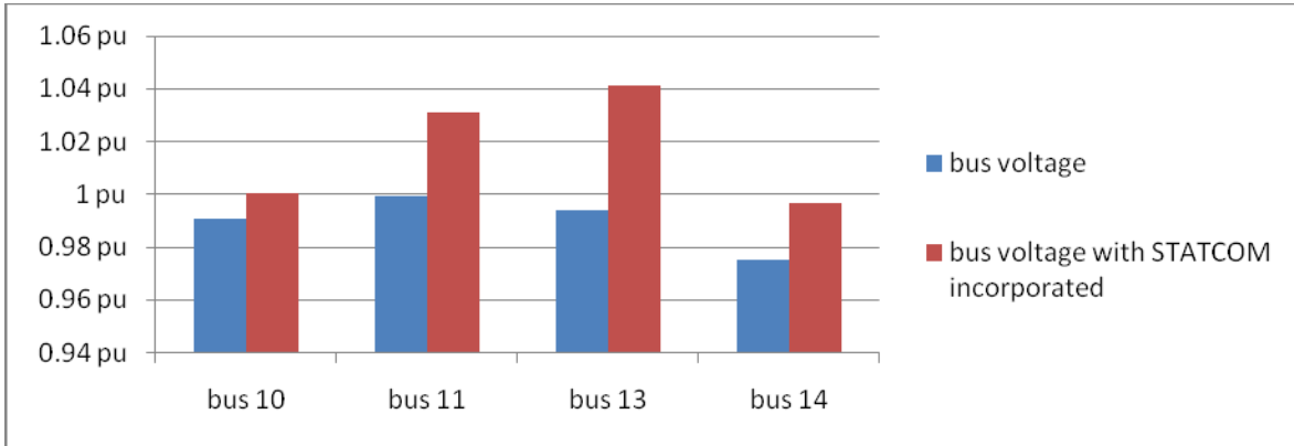
Fig 4 Graphical Representation of Improved Voltage Profile with STATCOM (IEEE 14 Bus)
