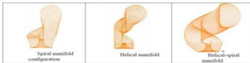
Figure 8: Modeled Spiral, Helical, Helical spiral manifolds
