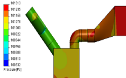
Figure 3. Bottom view pressure of AIS for without guide vane for 4000rpm [5]
