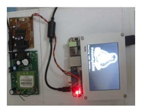
• Insert the SIM in the GSM Module.
