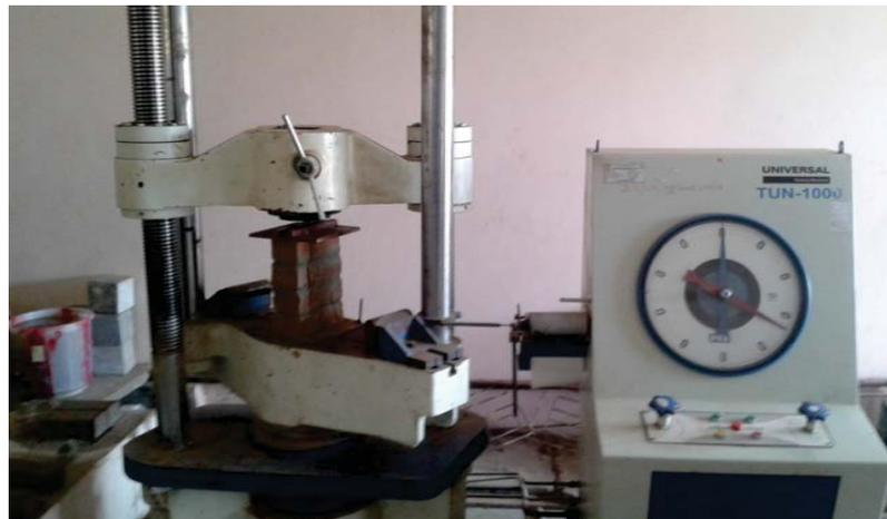
Fig11: Prism test
