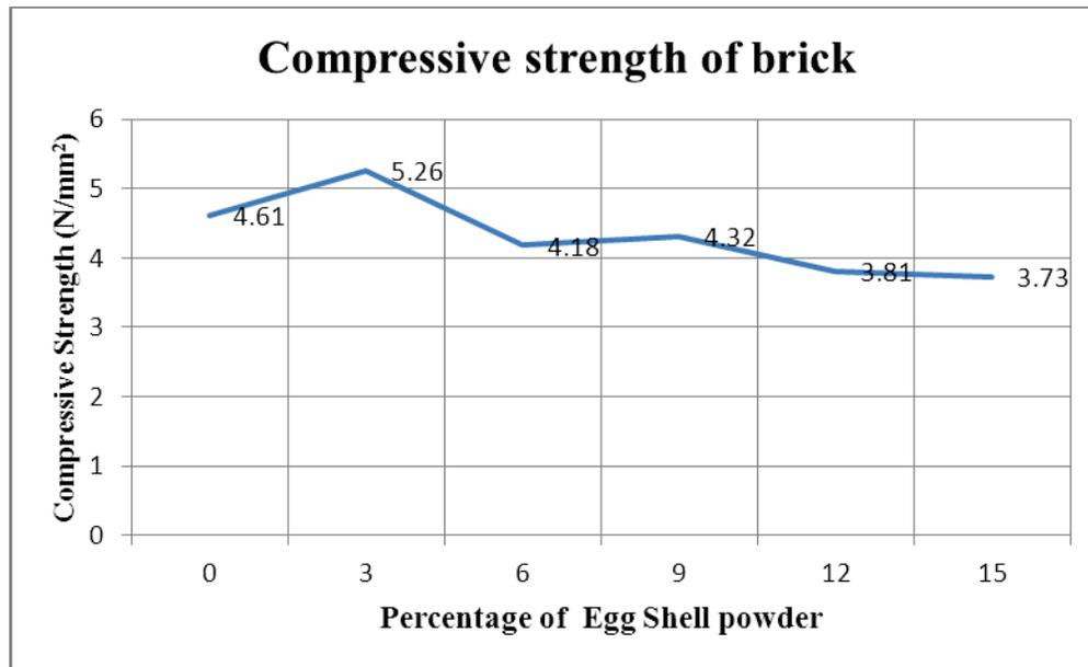
Fig8: compressive strength of bricks with respect to variation in ESP
