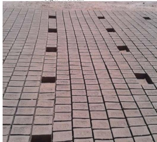
Fig6: Drying of bricks
