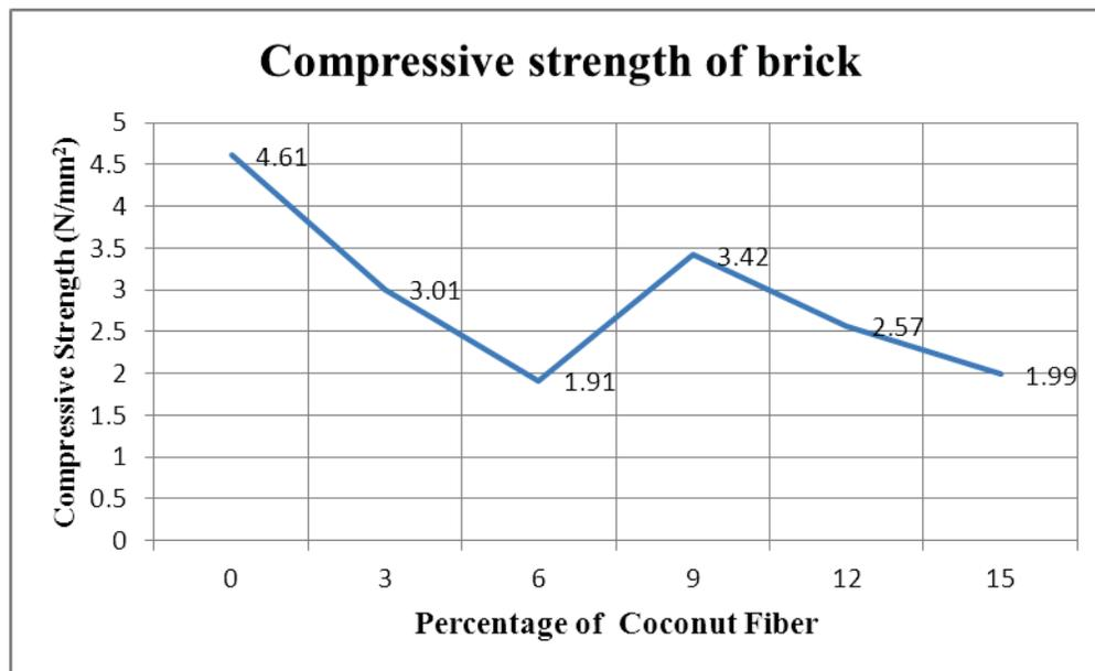
Fig9: compressive strength of bricks with respect to variation in CF
