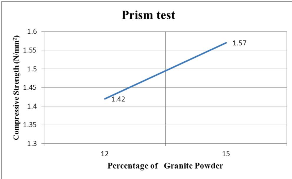
Fig10: compressive strength of bricks by prism test
