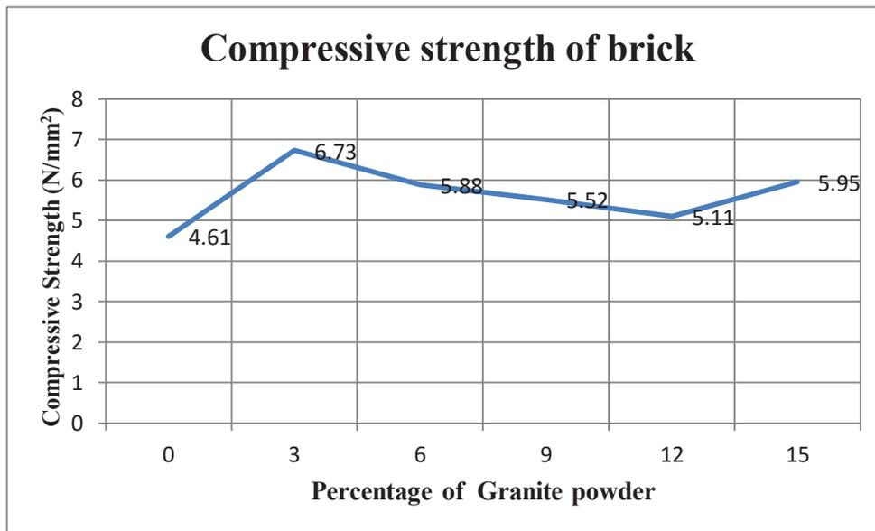
Fig7: compressive strength of bricks with respect to variation in GP
