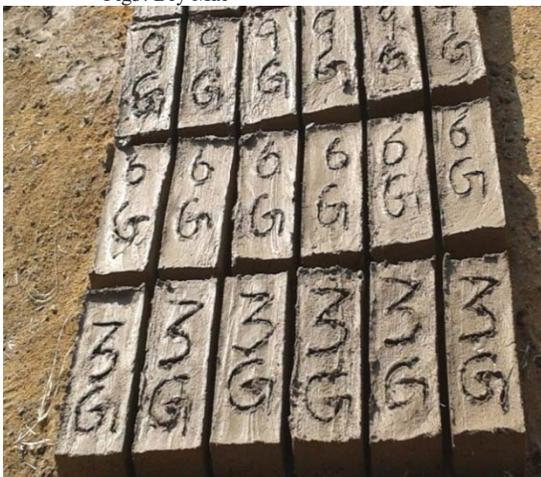
Fig5: Casting of bricks
