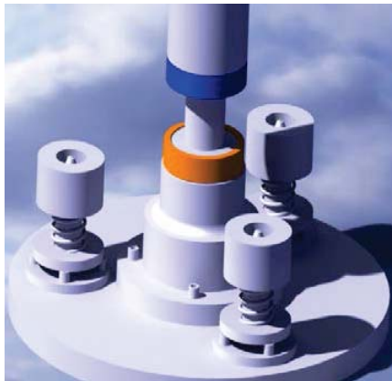
Figure 21: placement of raceway in the fixture Figure 22: assembling the inner hub on the fixture by placing raceways
