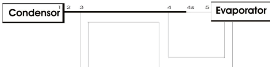
Fig. 2.2 Schematic diagram of capillary tube-suction line heat exchanger
