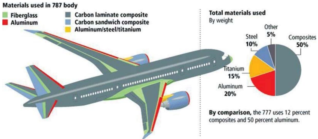
Fig.2 Materials used in 787 Body
