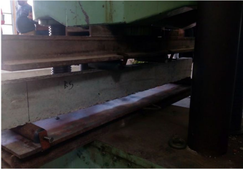
Fig.6 Loading Arrangement of tested beams
