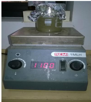
Fig 2.1 dissolving \text{AgNO}_3 in water by stirring
