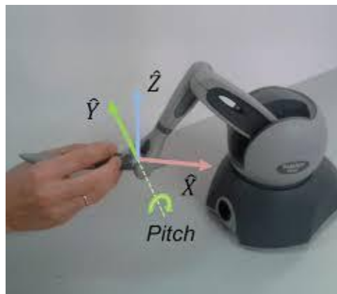
Figure 4. PHANToM haptic device with directions
