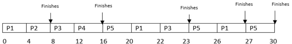
Figure 6. Gantt chart of IRR Algorithm
