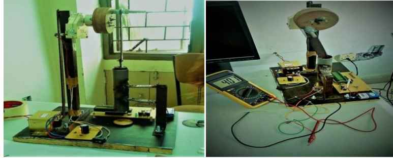
Fig: 1 Mechanism To Apply Periodic Dynamic Load On PVDF
