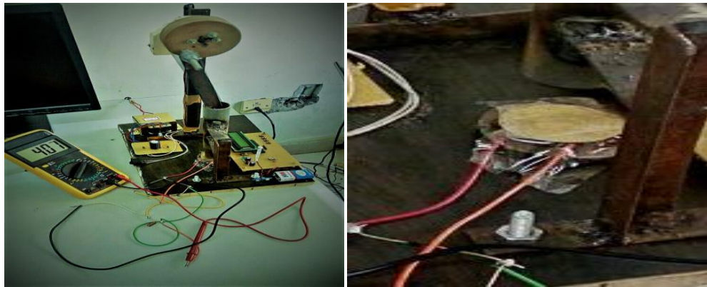
Fig: 10. Single Piezoelectric Full Wave Rectifier Circuit With Fixed Supported Boundary Condition
