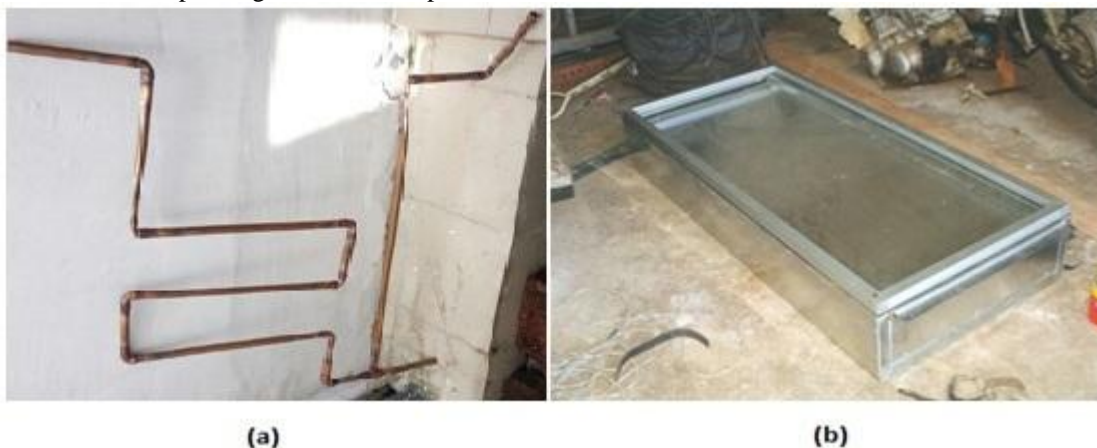
Figure-5.1: (a) Copper heat pipe exchanger (61 inch) and (b)Aluminum Container for PCM Composite (14x7 inches).
