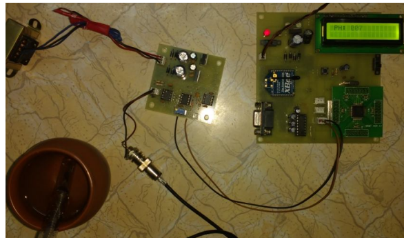
Figure6. Sensor Node unit measuring pH of water
