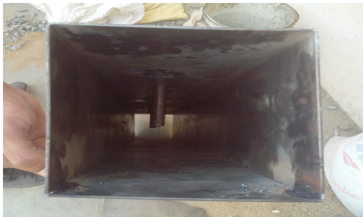
Fig2: Column with connectors (Column 2)
