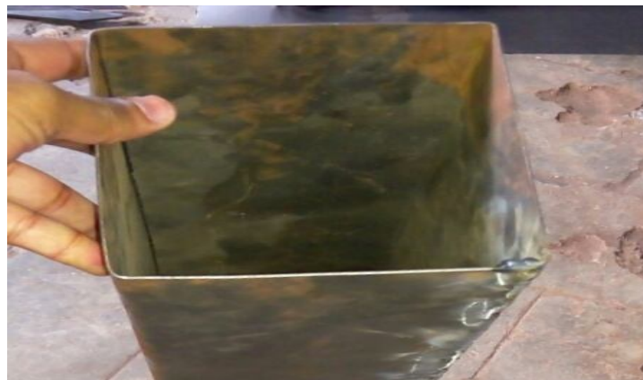
Fig3: Column without connectors (column 1)
