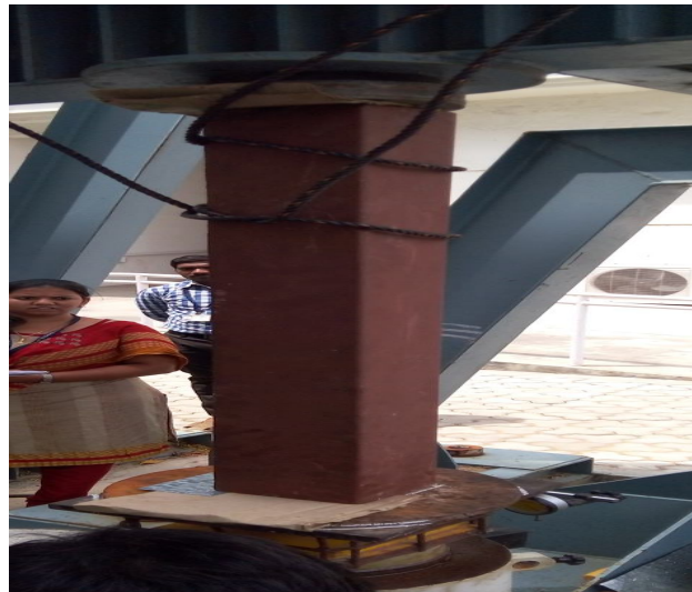
Fig10: Axial load testing of column
