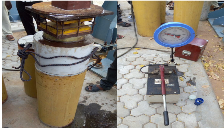
Fig 7: Application of loading from bottom with hydraulic jack
