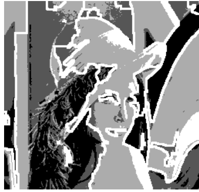
Figure 3.f Markers and object boundaries Superimposed on original image
