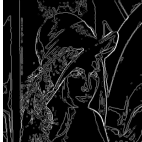
Figure 3.d Image produced by Marker Controlled Watershed Method
