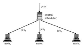
Jobs are first sent to the central scheduler, which then sends the jobs to the appropriate nodes. The jobs that cannot be started on a node are stored in a central job queue for a later start.
