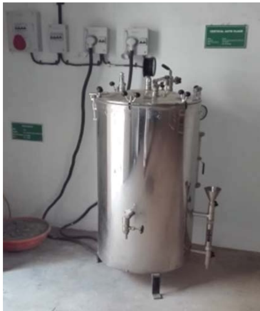
Fig 2 Steam Curing Process
