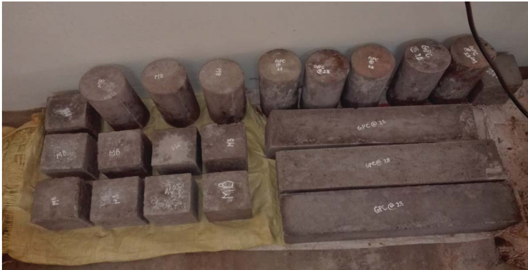
Fig 1 Specimens are casted in Geopolymer concrete using 8M and 12M
