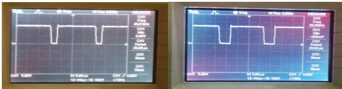
Figure14 above shows during hardware implementation gate pulses for switch S2 and S1 respectively.
