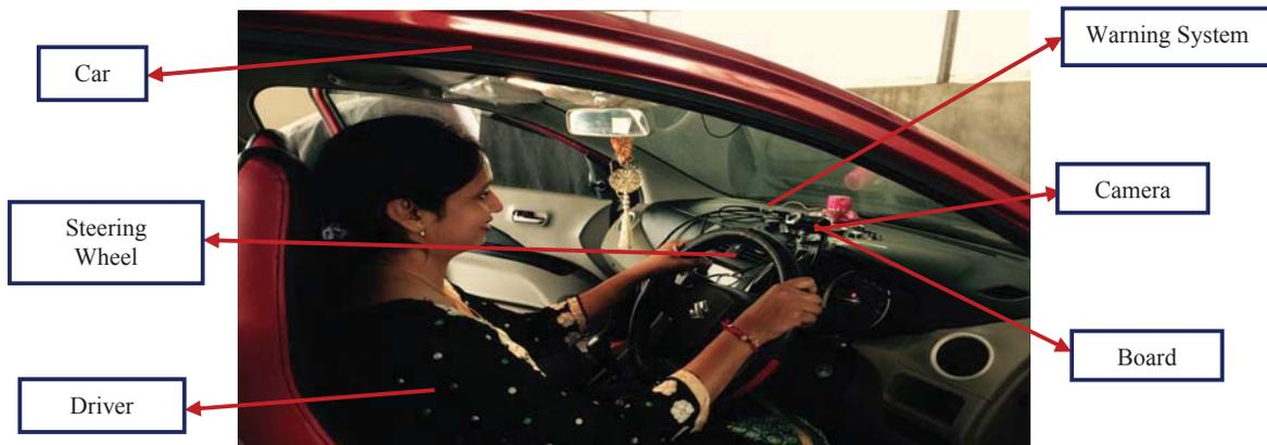
Figure 3: Real Time Implementation of HPLP Fatigue Detection System
