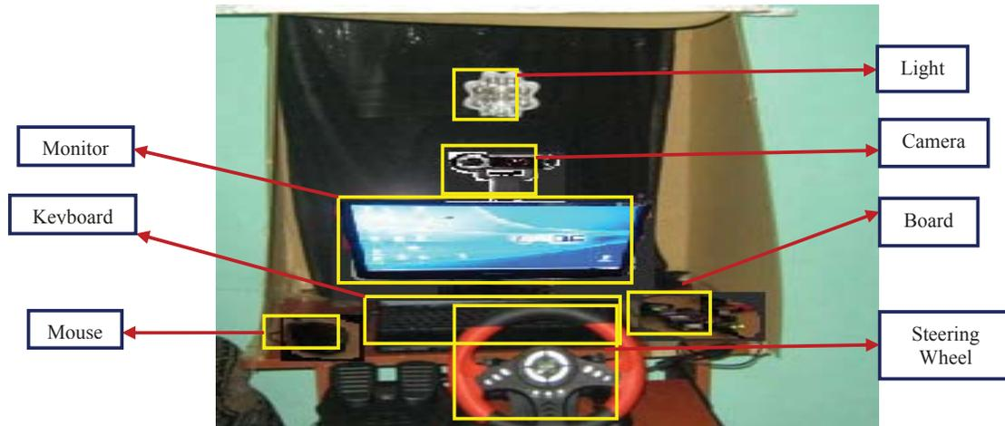
Figure 2: Prototype of HPLP Fatigue Detection System
