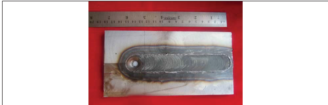
Figure 2a: Fabricated joint using FSW process
