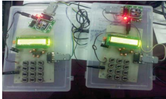
Fig: 5. Indexed 2.4GHz SIMO Transceiver implementation set
