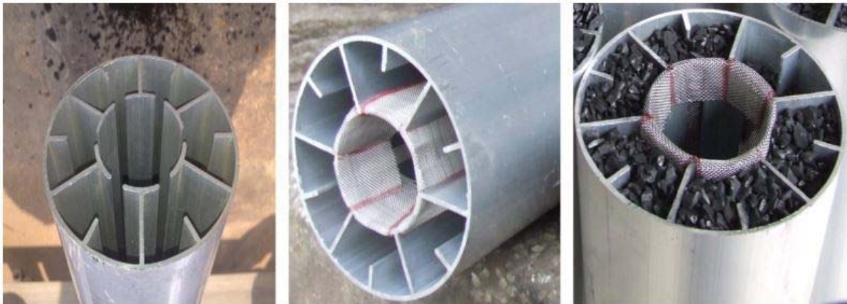
Fig. 8 – finned tube filled with Activated carbon [22].
