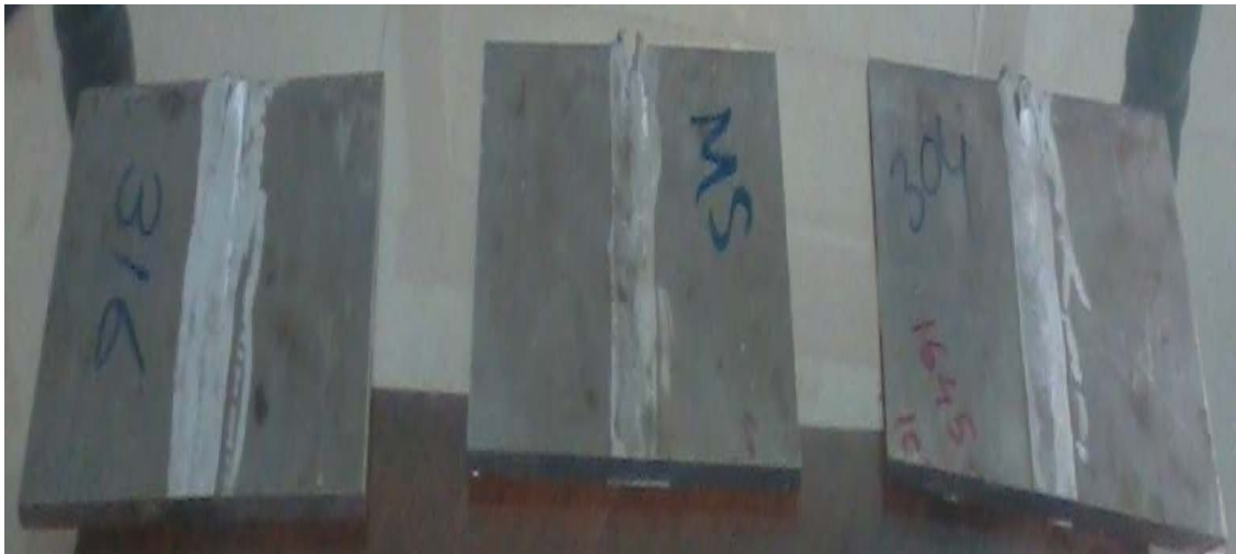
Figure 1: FSW Welded joints using 3 different tools
