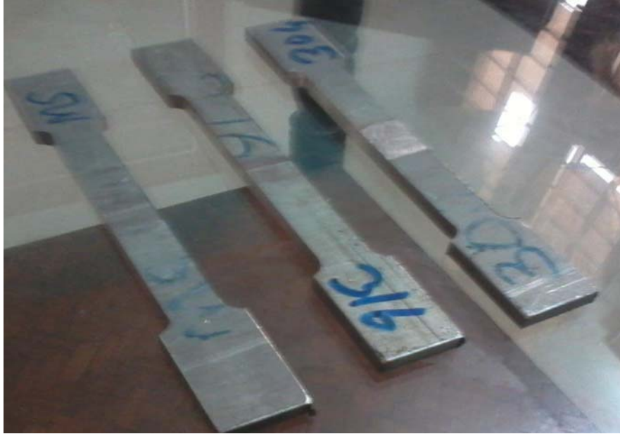
Figure 4: Tensile test specimens of FSW Welded joints using 3 different tools
