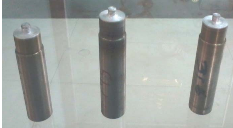
Figure 2: The three different tools used for FSW (SS 316, SS 304, and MS)
