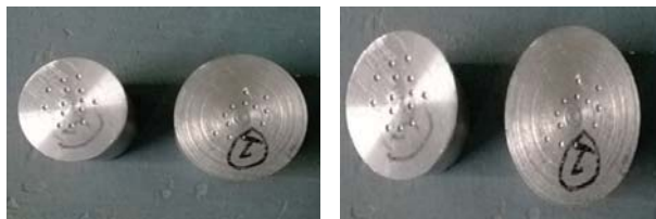
Fig.7 RWH Hardness test of Al 6061 and Al 6061/SiC
