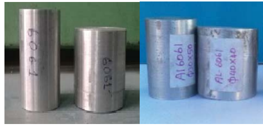
Fig.-2 Fabrications of Al6061 and Al6061/SiC different different cylindrical specimen
