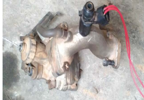
Fig: - 2 Carburetor with Injector
