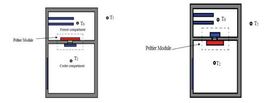
Figure 3 Experimental setup in Structure I with standalone VCR
