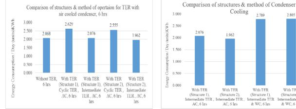
Figure 6 Energy Consumption with different methods with Air cooled
