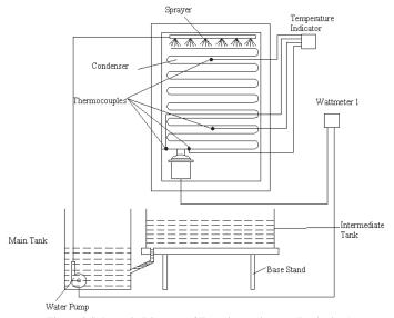
Figure 2 Schematic Diagram of Experimental setup (Back view)
