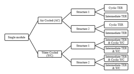
Figure 5 Experimentation methods for single TE module
