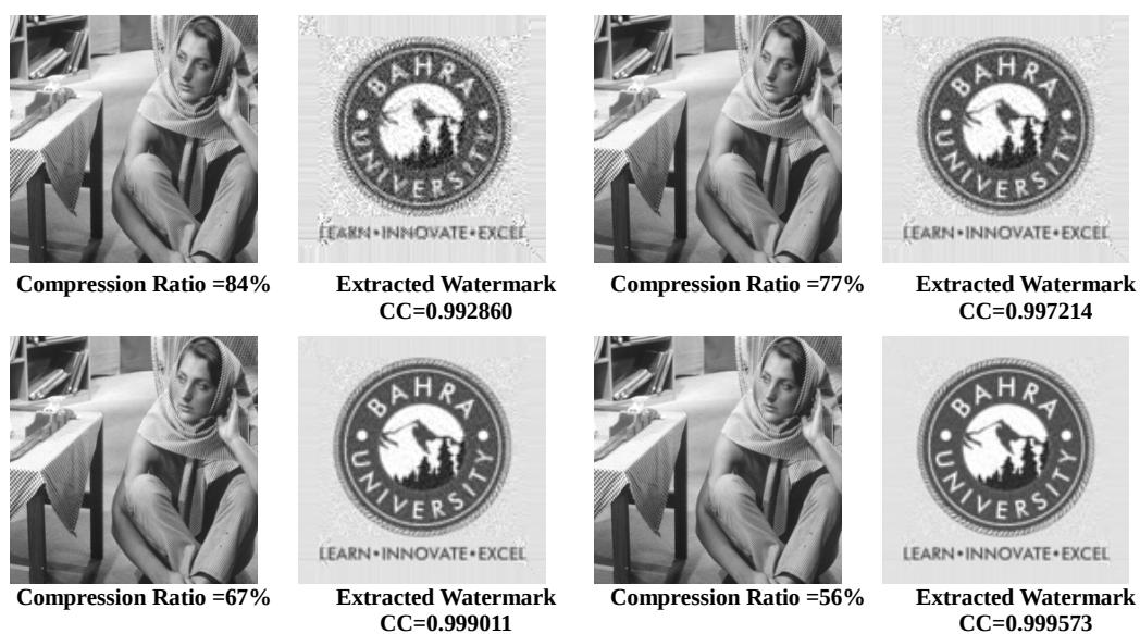
Figure-5: Results of watermarking by proposed DWT-SVD technique after salt & pepper noise attack
