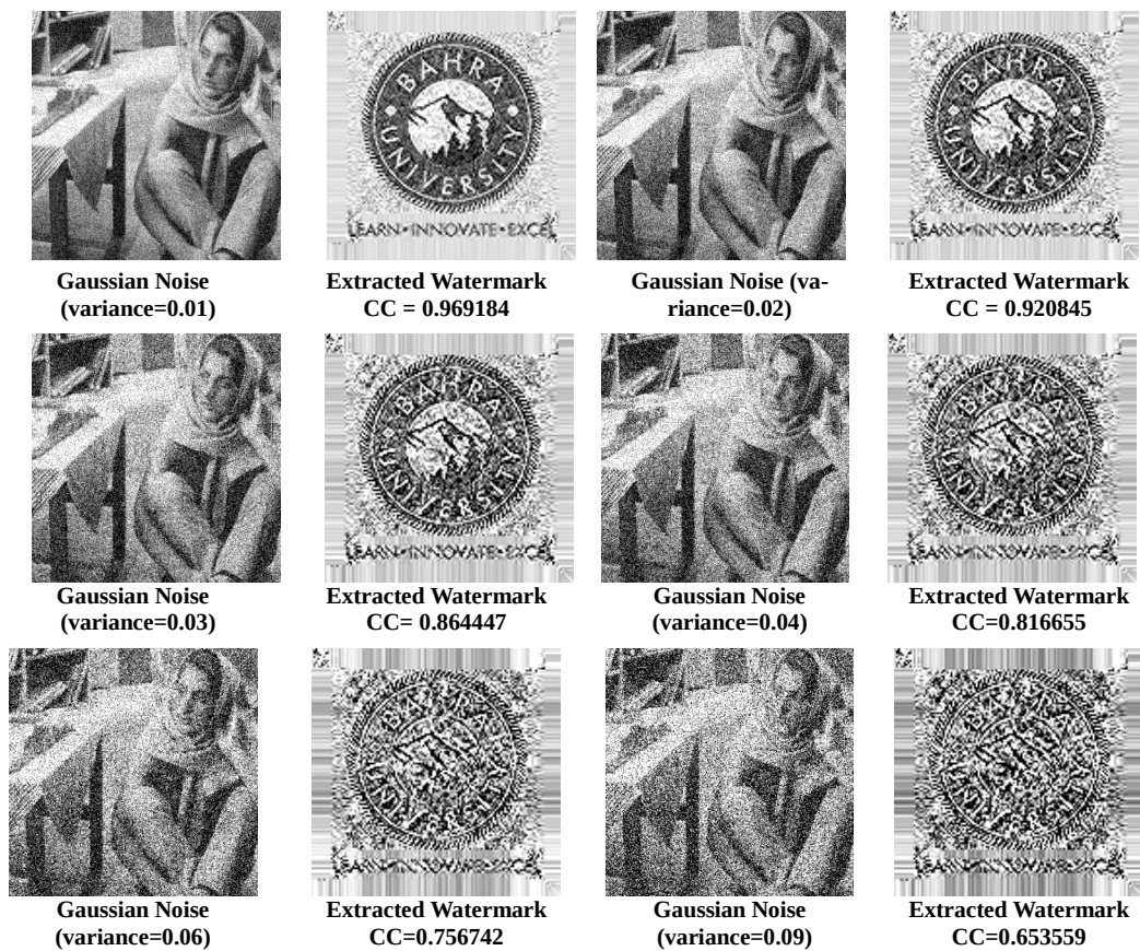
Figure-3: Results of watermarking by proposed DWT-SVD technique
