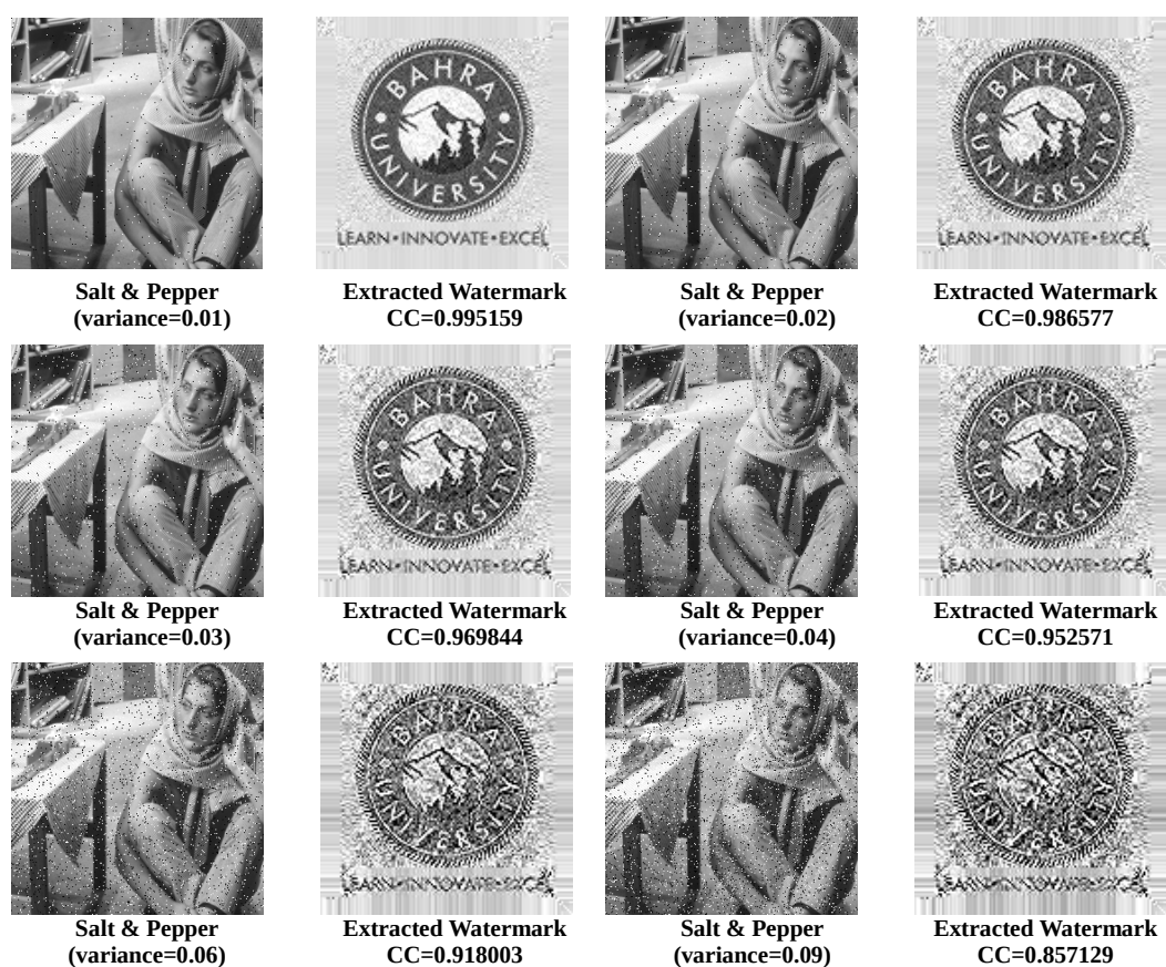
Figure-5: Results of watermarking by proposed DWT-SVD technique after salt & pepper noise attack
