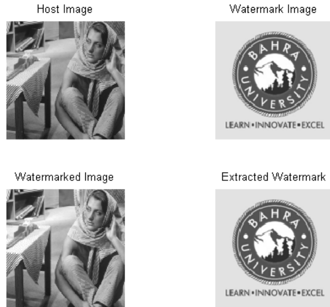
Figure-3: Results of watermarking by proposed DWT-SVD technique
