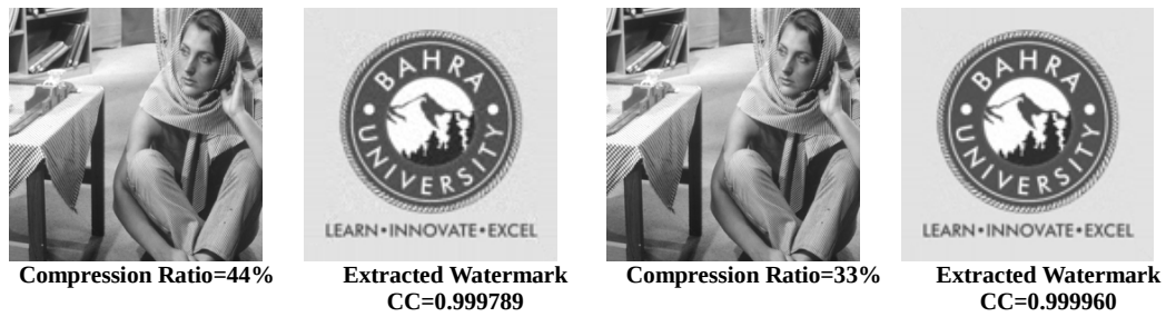
Figure-6: Results of watermarking by proposed DWT-SVD technique after DCT compression attack
