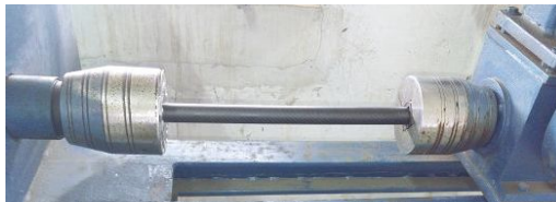
Figure 2. Torsional Testing of Carbon fiber composite shaft
