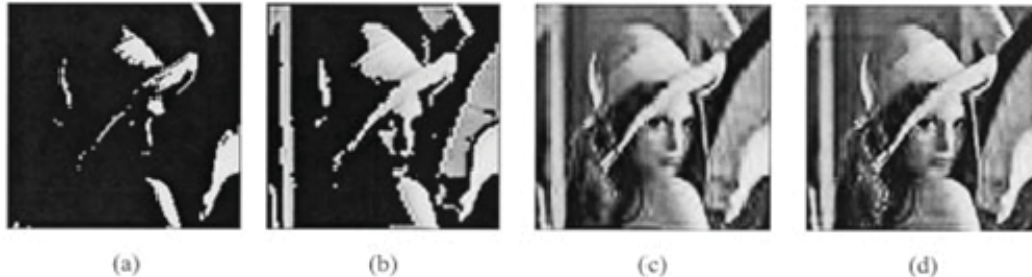
Figure 5. Reconstructed image Lena; DW-5; CR = 50 : 1. (a) J = 1 (PSNR = 8.40 dB). (b) J = 2 (PSNR = 11.76 dB). (c) J = 3 (PSNR = 23.39 dB). (d) J = 4 (PSNR = 24.40 dB).
